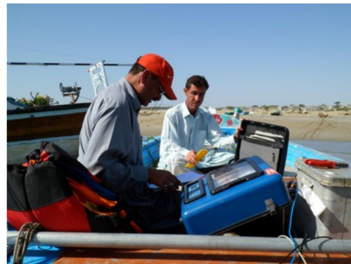
Bathy 500 Echosounder being used in bathymetric survey.
