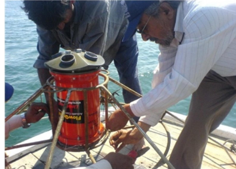
Acoustic Doppler Current Profiler (ADCP) being moored during survey.
