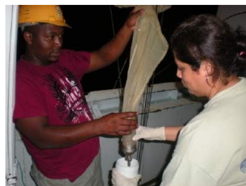
Plankton nets for sampling phytoplankton and micro-zooplankton during the November 2010 cruise.
